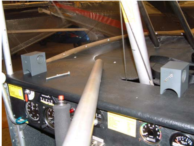
Figure 5; inner end of starboard wing support rod.
