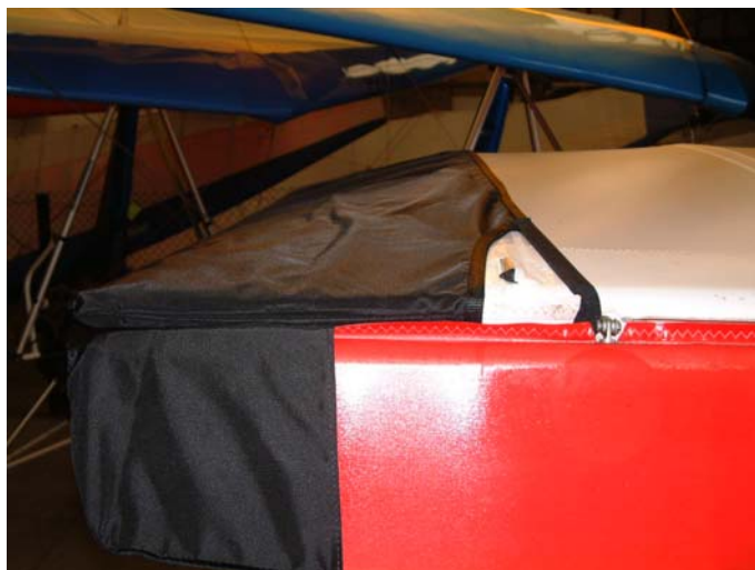
Figure 11; rear edge of wing-tip cover.
