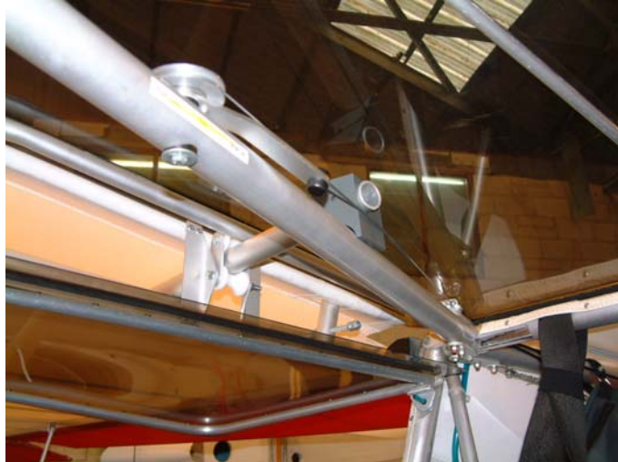
Figure 8; pull the rod back through the locating block in position on the cabin tube.
