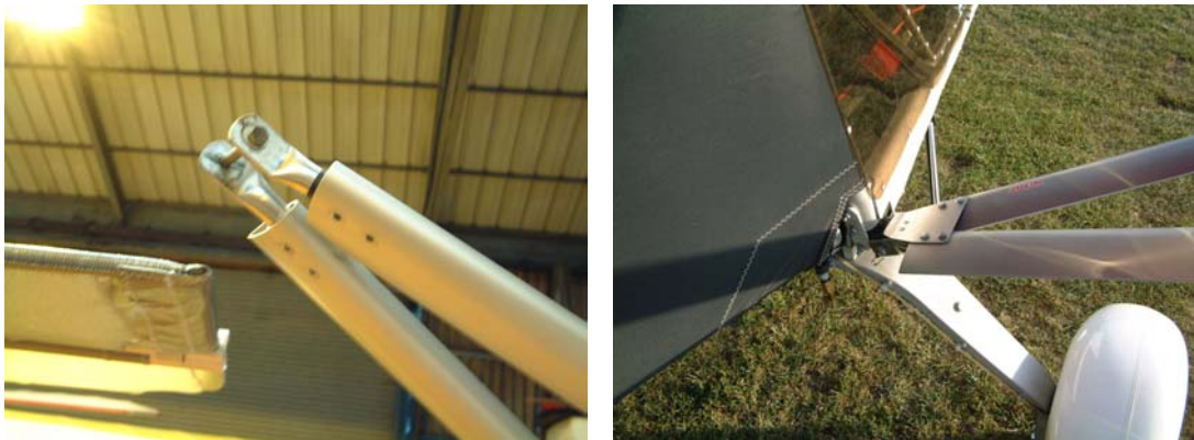
Figure 19; ready to fit lift strut plates, and fitted plate.
