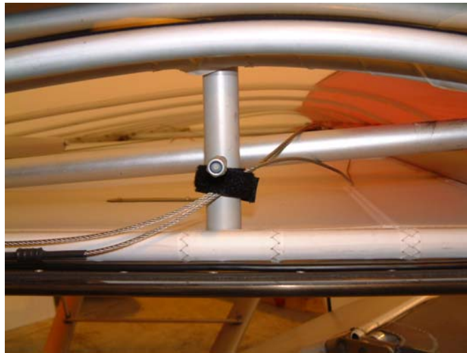
Figure 13; Velcro cable holders.
