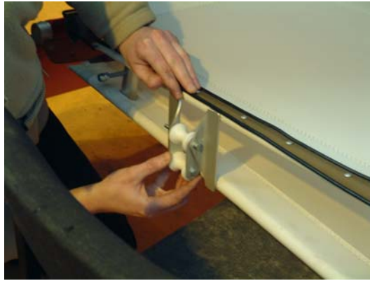
Figure 16; position the roller assembly on the wing root.
