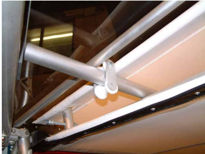
Figure 6; rollers loosely positioned.
