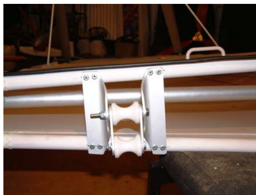
Figure 18; fully fitted wing roller assembly.
