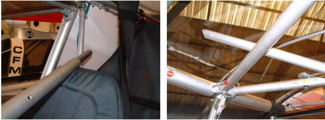
Figure 3; port rod inner end behind starboard door, then lift outer end up between cabin tubes.
