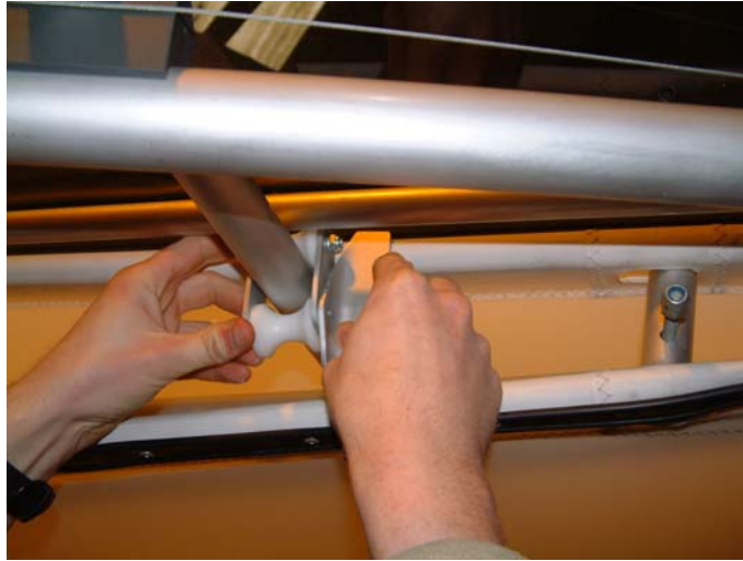
Figure 10; side plate measured to cut to length.
