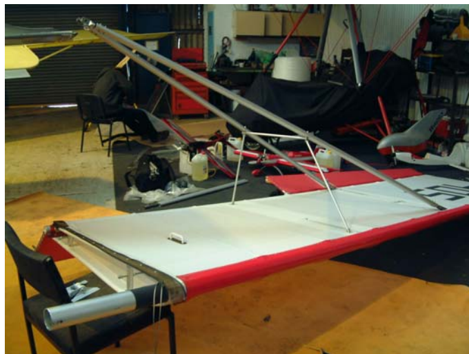
Figure 15; lay the wing down, propped up at the root on a chair or similar.
