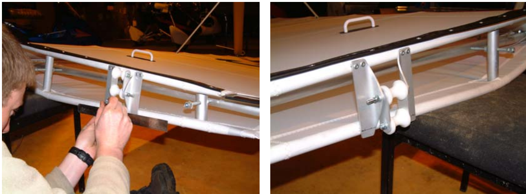
Figure 17; mark the rivet hole positions on the upper wing root batten (the wing is upside down).
