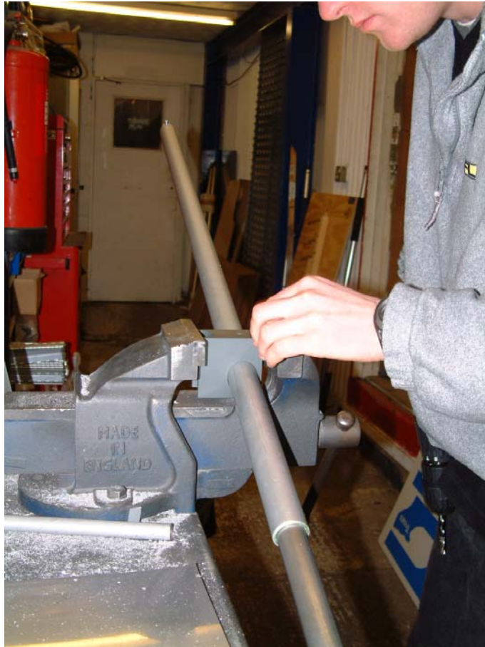
Figure 22; clamp tube and block in vice.
