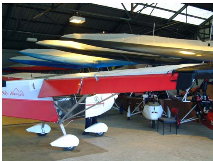
Figure 12; drooping ailerons and flaps.
