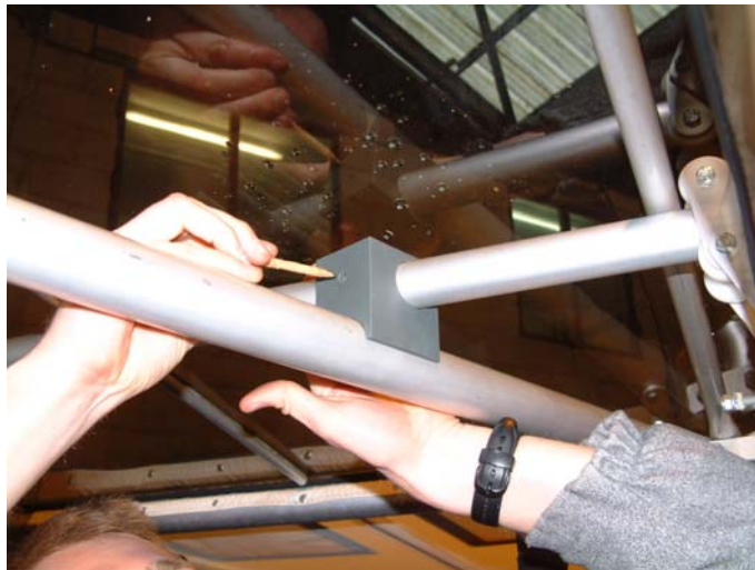
Figure 21; mark the holes with a slim pencil.
