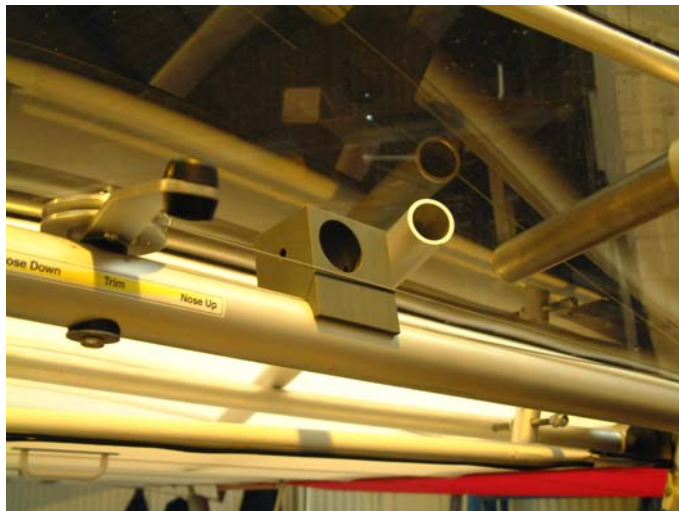
Figure 7; starboard locating block between trimmer cables.
